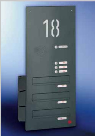
Fig. 5/3 Box format 300 x 110 x 265 - 410 mm, hinged steel front plate with RS1001 radius-profile closing frame with optional engraving. Letter plates 265 x 33 mm.
