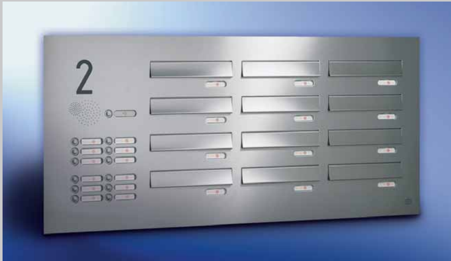
Fig. 5/1 Box format 300 x 110 x 385 mm, 24 mm front plate, with thermal break for mounting in door profile, with RSA , completely manufactured from V4A stainless steel. Letter plates 265 x 33 mm.
