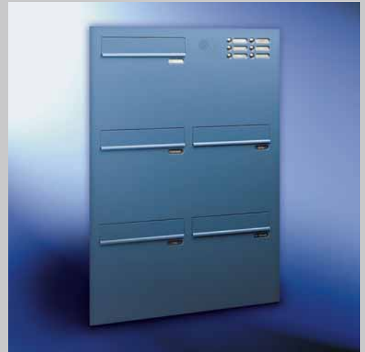
Fig. 5/2 Box format 370 x 330 x 145 mm, with RS50 , 24 mm steel front plate, with thermal break for mounting in door profile, with RSA . Letter plates 335 x 50 mm.
